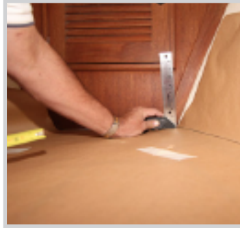
6 - In order to make the mattress edges follow the outward shape of the hull, you need to measure the Beveled or Tapered Edge.
