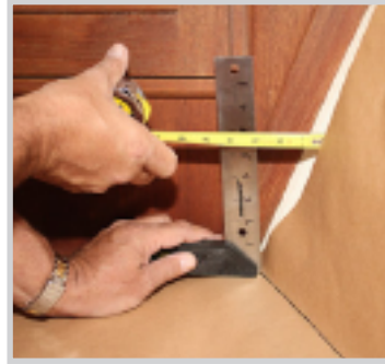
7 - Measure the distance between the square and hull. Based on the thickness of the mattress you have chosen. Example: If you have chose the 6" Latex go up 6" on the square and measure across to hull.
