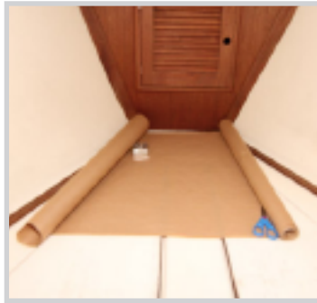
2 - Roll Out Paper across Narrow End or Bulkhead.
